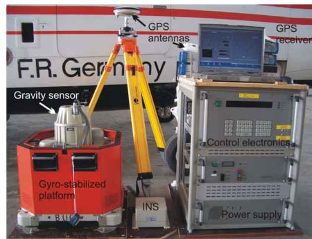
Fig. 1 Aerogravity system consisting of the KSS31M gravity meter (platform with sensor and electronics rack), GPS instrumentation, INS unit and laptop.
