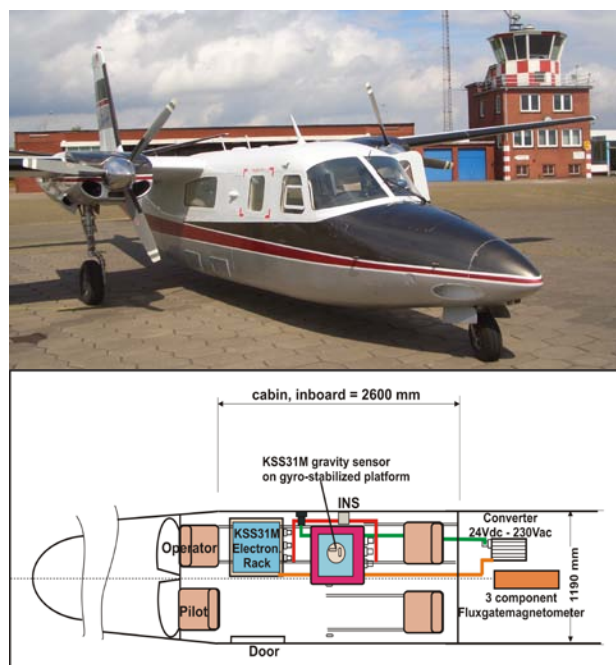
Fig. 2 Aero Commander 680 FL of Air Tempelhof (above). System installation in the aircraft cabin is shown below.
