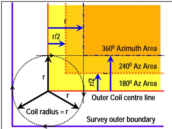
Figure 2a: Coverage areas for a coil survey.
