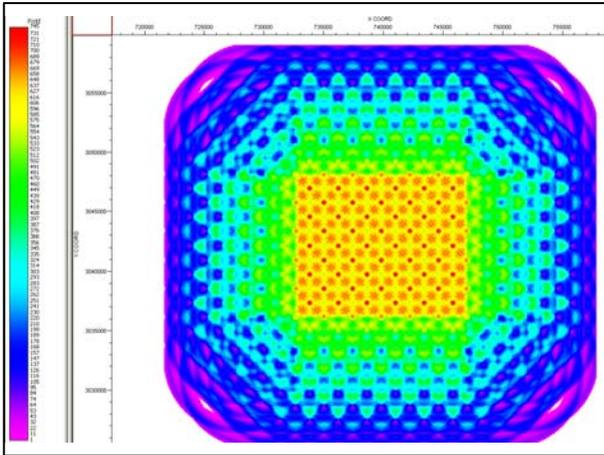
Figure 3b: Corresponding coil surveys fold of coverage.
