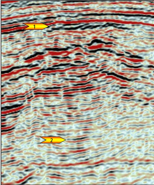
Figure 5a: A narrow-azimuth seismic section taken from an underlying 3D survey. Arrows 1 & 2 highlight remnant multiple energy contaminating the narrow azimuth image not evident on the coil image.
