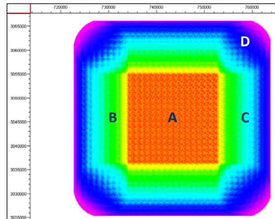
Figure 1a: Fold and offset/azimuth distribution for a high effort coil survey.
