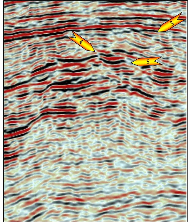
Figure 5b: A coil seismic section taken from the 3D coil pilot survey. Arrow 3 highlights dipping primary energy. Arrow 4 highlights better fault definition. Arrow 5 highlights improved imaging of primary reflections. All illustrate imaging benefits of coil over a narrow azimuth acquisition configuration.
