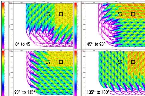
Figure 4: Number of populated offsets for four azimuth groups.
