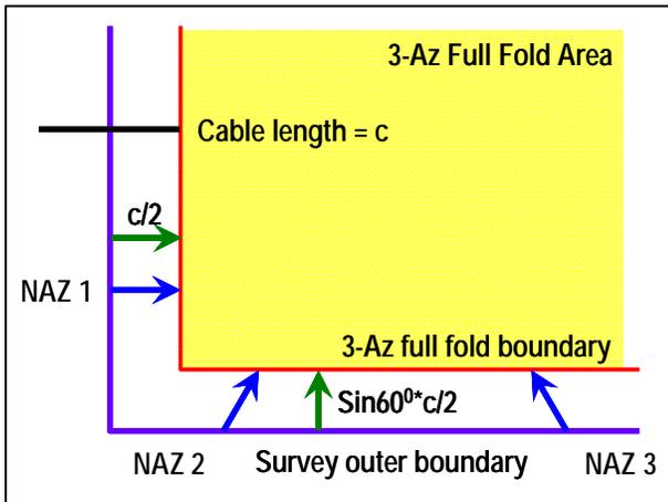
Figure 2b: Coverage areas for a three-survey narrow azimuth.
