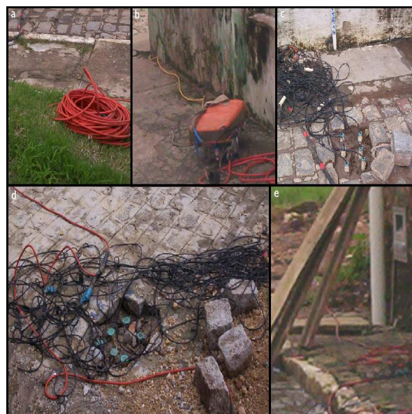
Figure 4 – Recording of data in the city of Rosário do Catete: a – Seismographic cables; b – Communication boxes; c e d – Geophone arrays; e – Cables.
