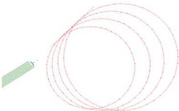
Figure 11: Coil shooting feasibility test: four circles with radii of 5.5, 6, 6.5, and 7km were shot
