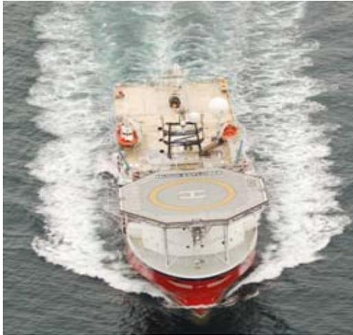
Fig. 3: The Hugin Explorer during the shakedown test offshore Norway. She has 500 ocean bottom nodes (OBN), Remotely Operated Vehicle (ROV), dual source, and a streamer.
