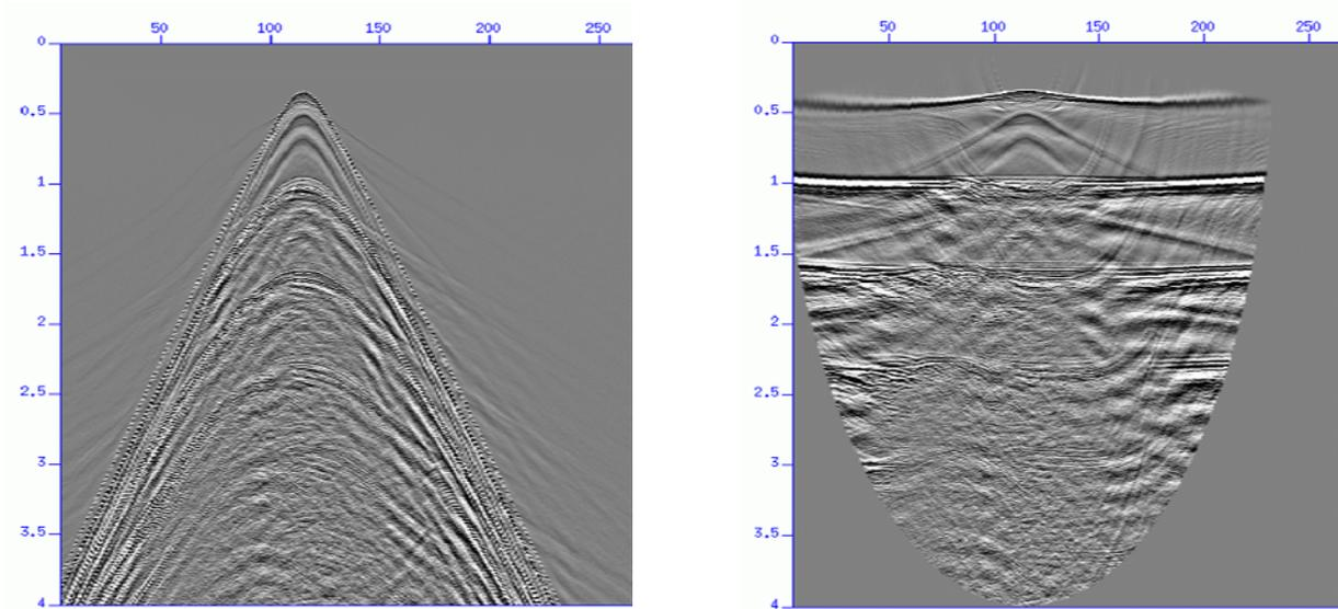
Fig 8. Common receiver gather before (a) and after (b) NMO with water velocity. Granite outcrop about 2 km away from the node is seen on the refraction in (a) and on the multiples in (b).
