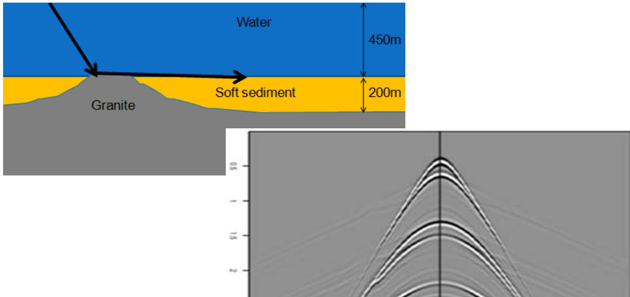
Fig 14. Details from Fig 12a. Granite outcrop about 2 km away from the node is seen on the refraction.
