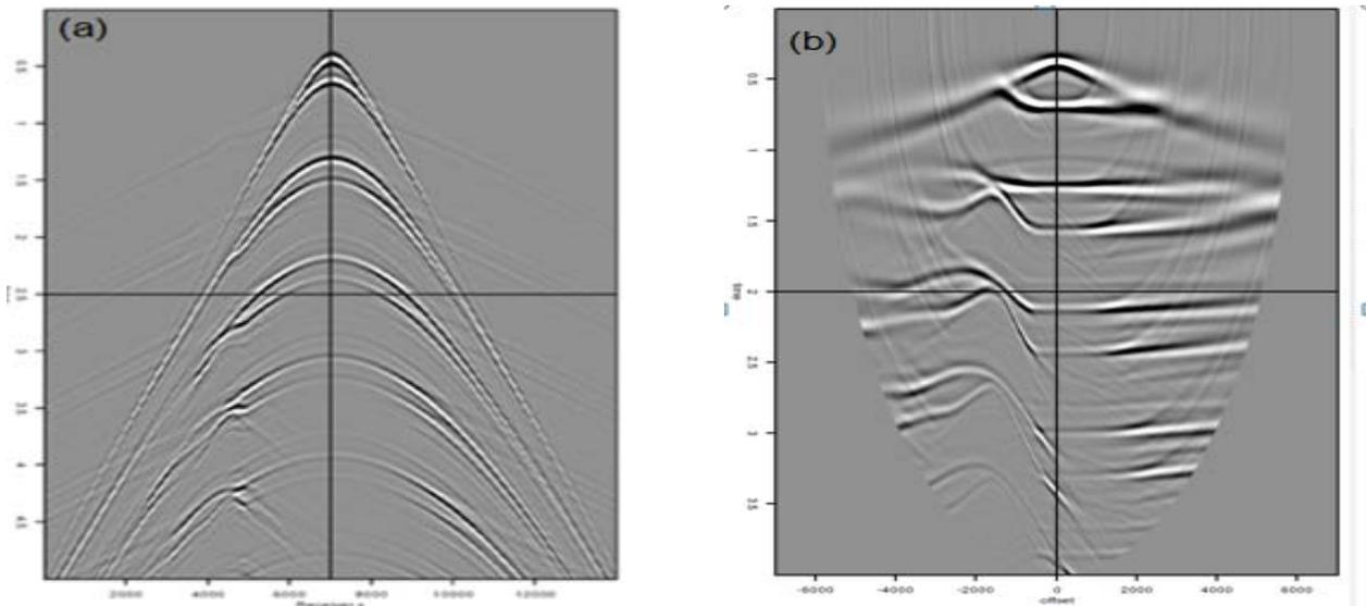
Fig 12. Common receiver gather before (a) and after (b) NMO with water velocity. Granite outcrop about 2 km away from the node is seen on the refraction in (a) and on the multiples in (b). Compare to Fig 8.
