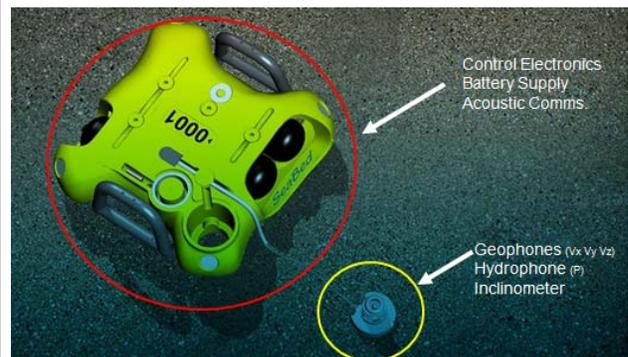
Fig. 2. Each ocean bottom node has an external planted sensor package containing a hydrophone and 3 geophones in vertical and two horizontal orientations.
