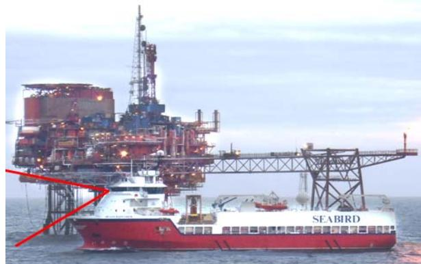
Fig 4b. The Hugin Explorer was designed to work safely in obstructed oilfields--the bridge is at the front and the helideck does not obstruct the view from the bridge.
