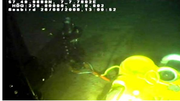
Fig. 6: ROV planting external sensor package during the shakedown test.
