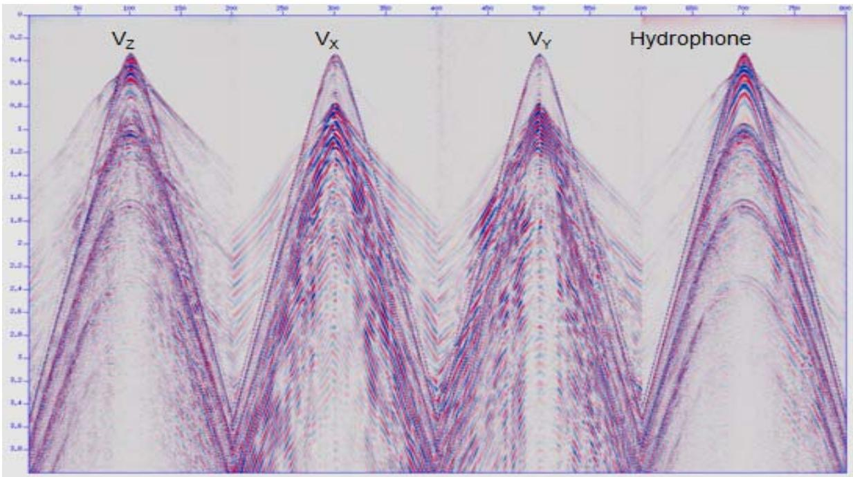
Fig 7: Shakedown test common receiver gather. 5km Offset. 50m Shot Interval. No Processing except gain. Note the P waves recorded on the Hydrophone and Vertical components and the shear waves recorded on the horizontal components  $V_x$  and  $V_y$ .
