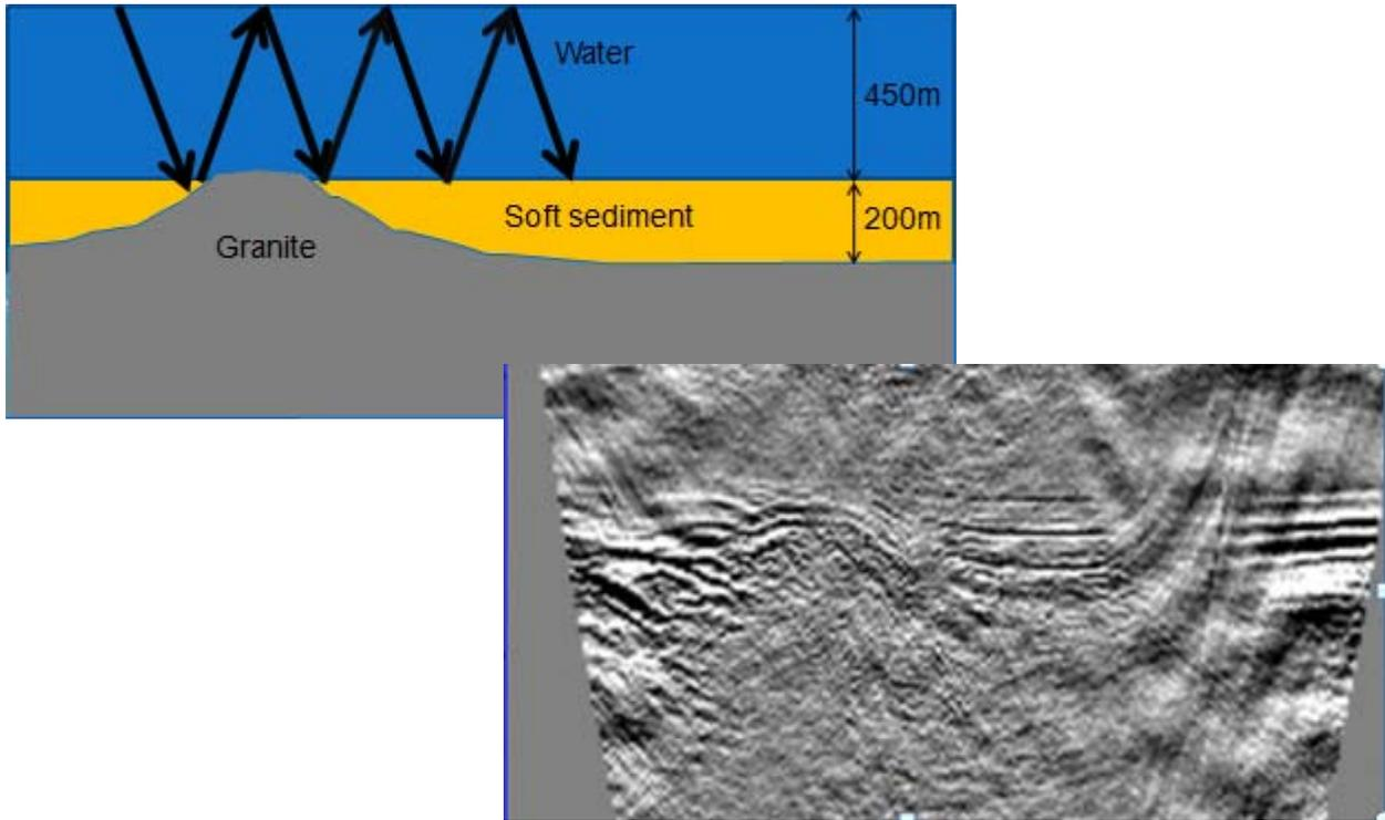
Fig 9. Details from Fig 8b. Granite outcrop about 2 km away from the node is seen on the multiples.
