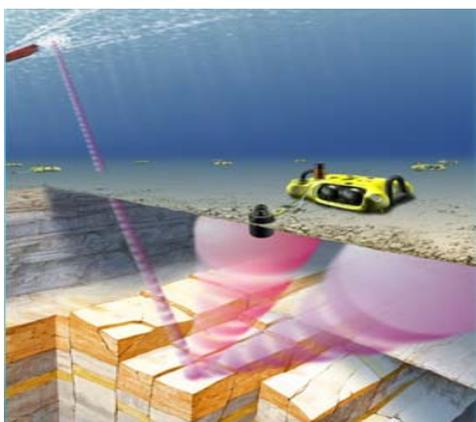
Fig. 1: Ocean Bottom Nodes recording reflections from geological formations and reservoirs. Some of the P waves emitted by the source are reflected as P waves and some are converted and reflected as shear waves. Note the sparse array of nodes on the seabed. The shot geometry, on the other hand, is dense.
