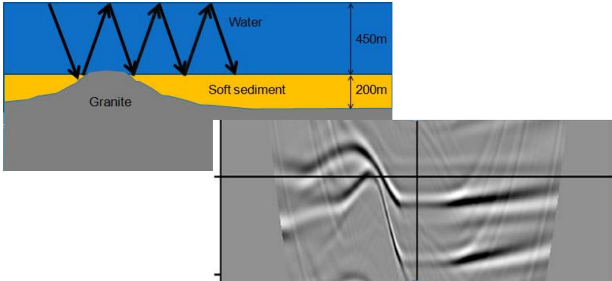
Fig 13. Details from Fig 12b. Granite outcrop about 2 km away from the node is seen on the multiples.
