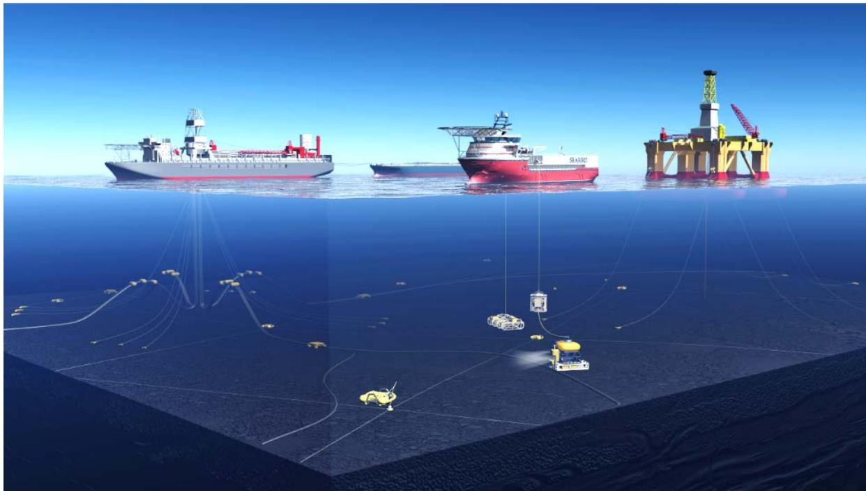
Fig 4a. Surface and subsea obstructions are no longer a major challenge in getting seismic over the reservoir with the use of ocean bottom nodes.
