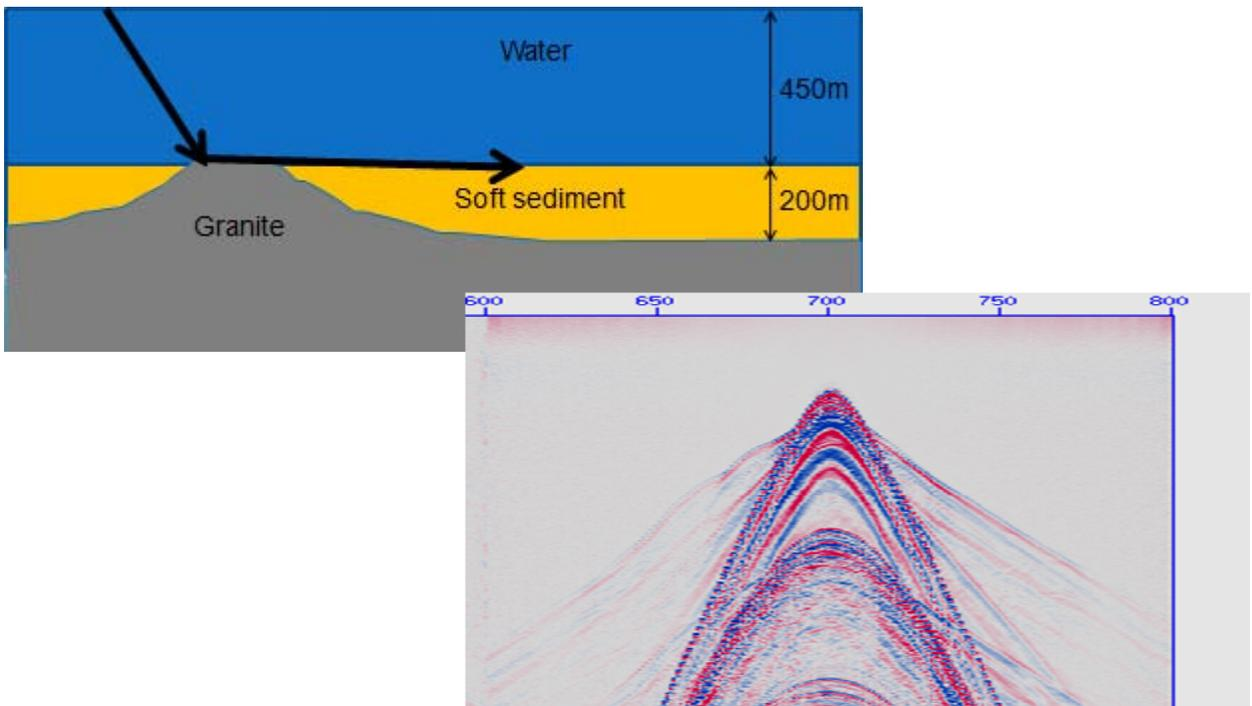
Fig 10. Details from Fig 8a. Granite outcrop about 2 km away from the node is seen on the refraction.
