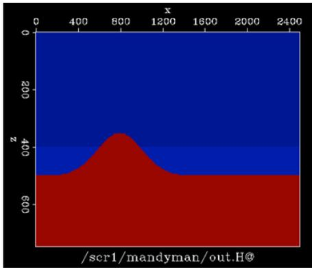
Fig. 11: Velocity model for wave equation finite differencing modeling.
