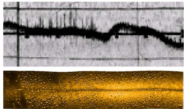
**Figure 2b:** Sonogram and echo sounder record showing isolated reef structures (P1).
