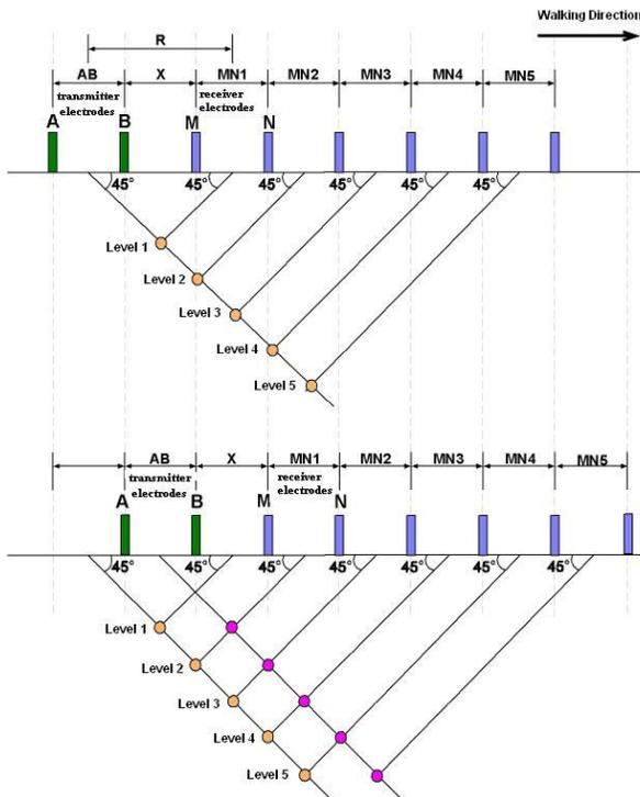
Figure 2: Layout of the electrodes arrange.
