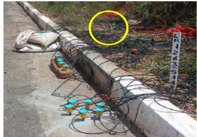
Figure 1: Geophone coupling test. The yellow circle shows a group of geophone coupled directly to earth.
