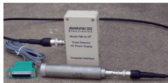
Figure 1: He-3 neutron tube detector and high voltage power supply used to monitor neutron flux.
