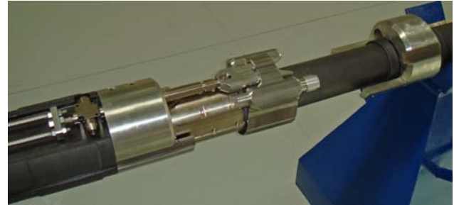
Figure 5: The clamping device in its closed state with a geophone mounted.
