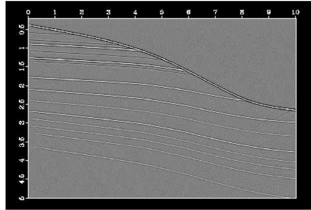
**Figure 5:** Zero-offset section generated by Kirchhoff modeling.
