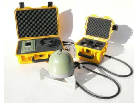
Figure 4: 3-component, high sensitivity broadband seismometers.
