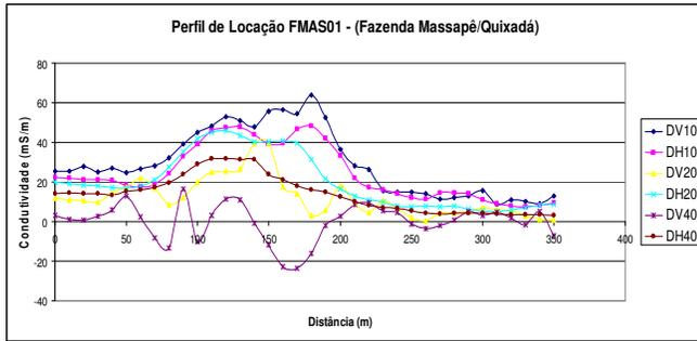
Figure 3 – EM34 Survey – Profile 01 with all Dipole modes.
