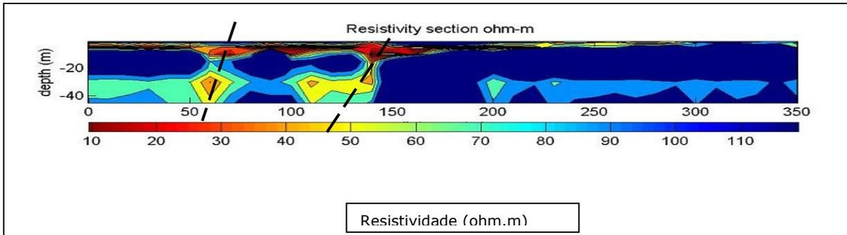
Figure 6 – Interpretation of Interpolated Quasi-2D Geoelectrical Model.
