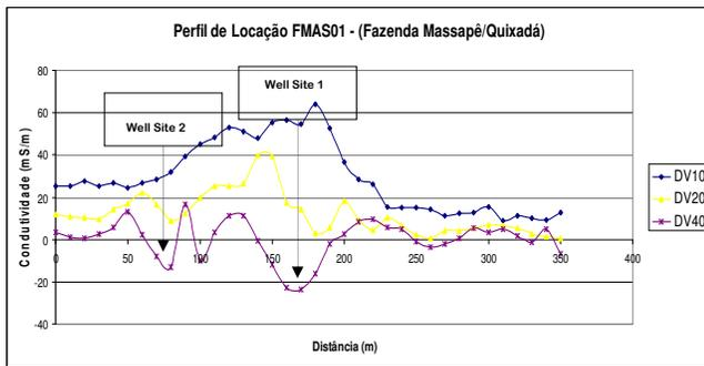
Figure 4 – EM34 Survey – Profile 01 with Vertical Dipole mode and Well Location suggested.
