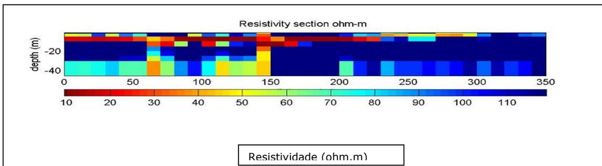
Figure 5 – Quasi-2D Geoelectrical Model.
