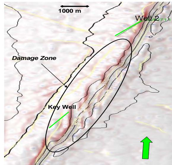
Figure 3: Minimum curvature map at Apon Formation, at northern of study area showing a damage zone (red lines inside black oval) along a sector the Lama – Icotea fault
