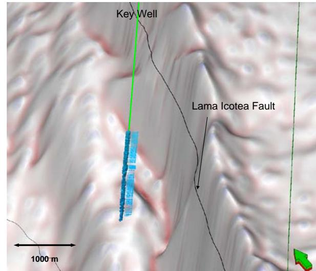
Figure 5: Fractures orientations (light blue circles) in the Key Well (light green line) associated with the 3D seismic interpretation from Curvature Attribute. Horizontal axis of Lama-Icoatea fault is represented by the black line.
