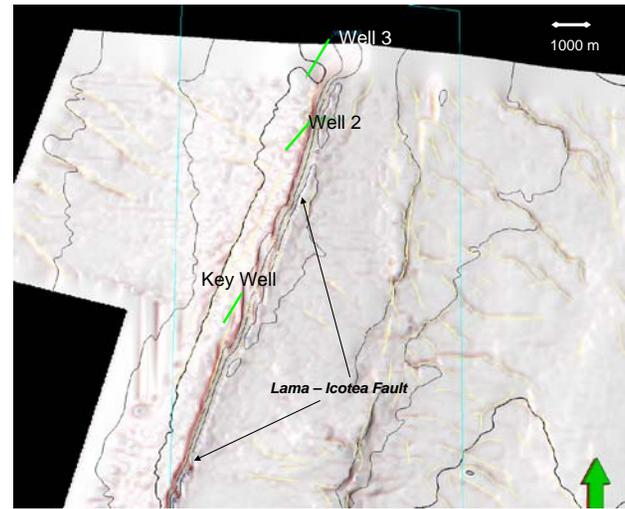
Figure 2: Minimum Curvature map (at level of Apon Formation) at northern of study area. Solid green lines represent three wells situated into the study area. Red trends shows are associated with the orientation of the mains faults systems (see Lama – Icotea Fault), and yellow lines are the fault polygons got from 3D seismic interpretation.
