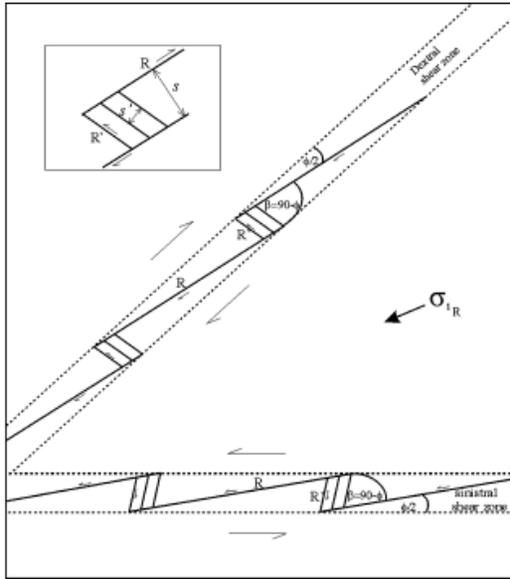
Figure 4: Basic Riedel shear structures forming sinistral and dextral conjugate shear-zones. R and R' are synthetics and antithetic shear bands,  $\beta$  is the angle between R and R' and  $\phi$  is the angle of internal friction.  $\Sigma_{1R}$  denotes the remote maximum compressive principal stress.
