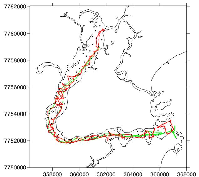
**Figura 1:** Study area showing samples location (black dots), sidescan sonar transects (green lines) and seismic transects (red lines).
