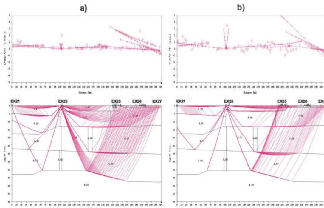
Figure 3 – Examples of: a) Travel-time curve and the ray tracing for P wave (speed reduction 6 km/s) b) travel-time curve and the ray tracing for S wave (speed reduction 3.46 km / s) (Perosi, 2006)
