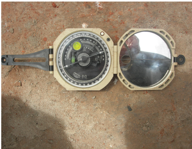
FIGURE 3: The compass showing the orientation of the seismometer to the geographic north with a magnetic declination on 20,5°.
