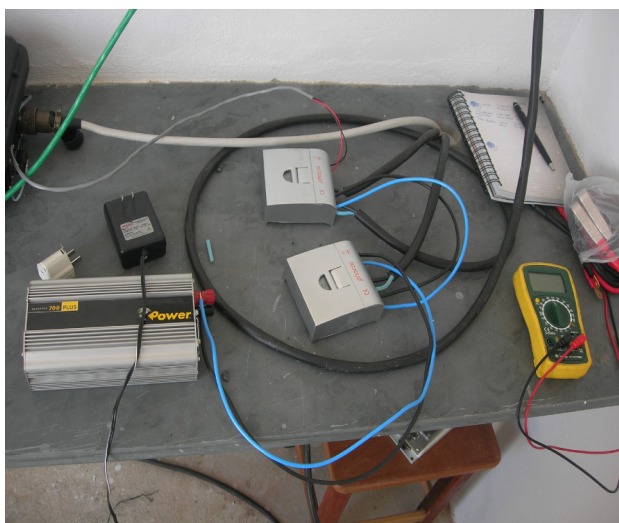
FIGURE 8: Electric circuit with the charge regulators.
