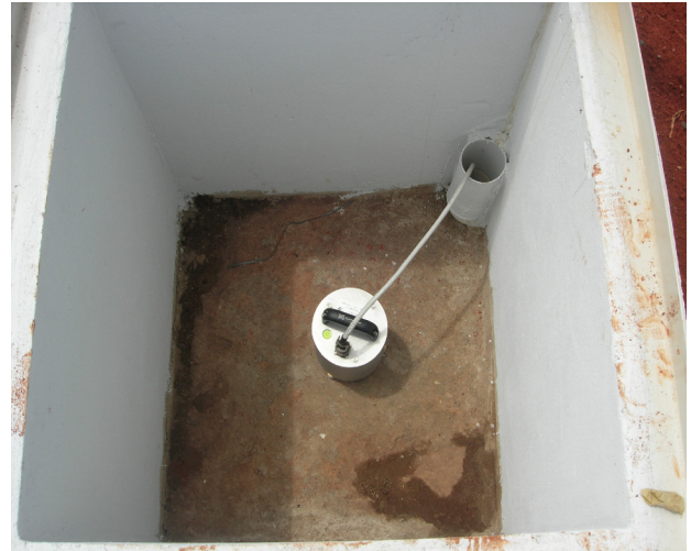
FIGURE 4: Installed seismometer (isolated, oriented and horizontally leveled).
