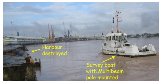
Fig. 2 – Bathymetric Survey close to the sunken pier in Itajaí harbor.
