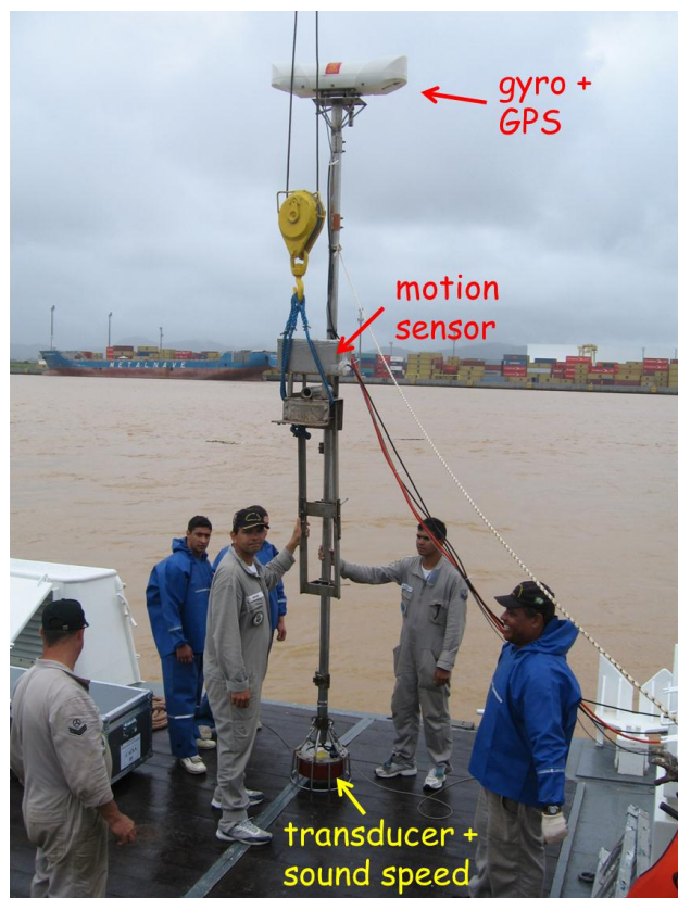
Fig. 1 – EM3000 multibeam sensors – pole mounted, ready to be installed in the survey boat (LB Betelgeuse).
