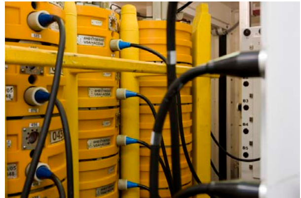
Figure 4: Z3000 nodes – Data unloading/charging
