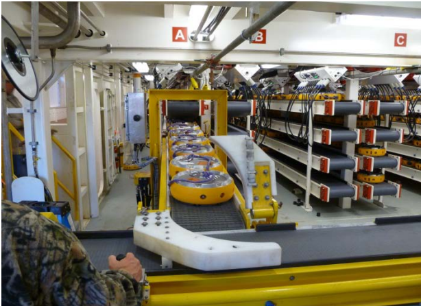
Figure 16: Node Handling Conveyor Belts Onboard
