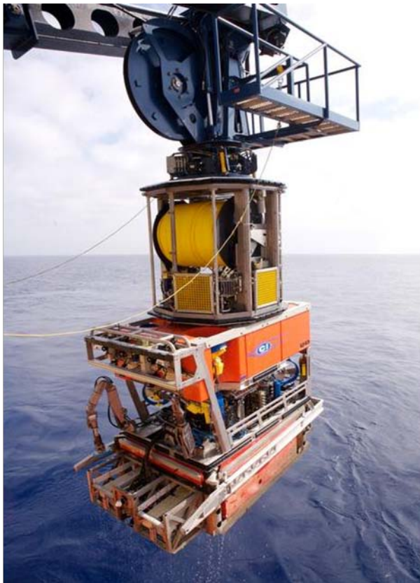
Figure 6: Schilling ROV, with under-slung node skid and Tether Management System (TMS)
