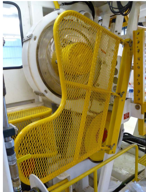
Figure 14: Custom design pinch sheave for node rope deployment and recovery
