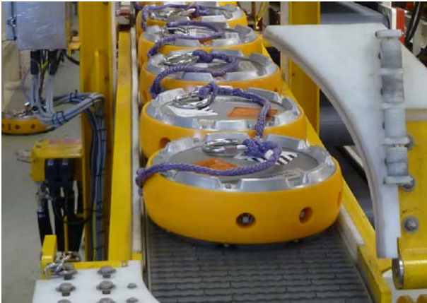
Figure 12: Z700 Nodes on conveyor belts used for onboard handling
