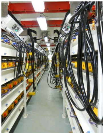
Figure 17: Node Charging/Synchronising/Data Unloading
