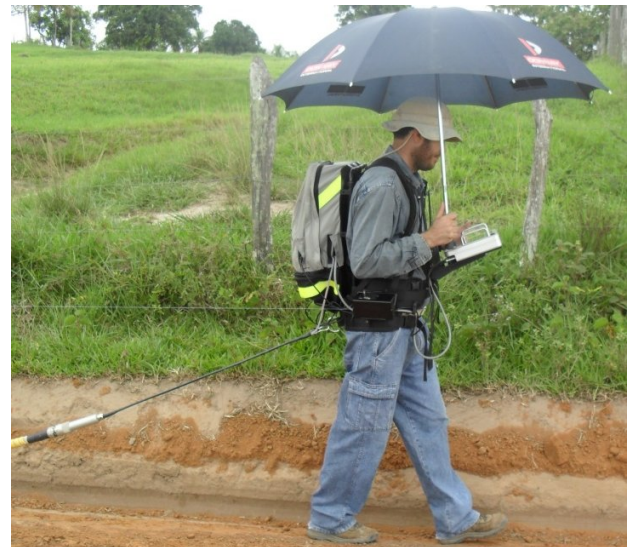
Fig 3 – GPR system employed in the survey.
