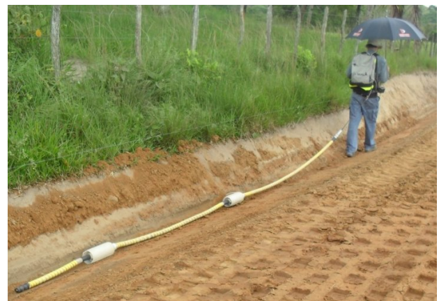
Fig 4 – Rough Terrain Antenna employed in the survey
