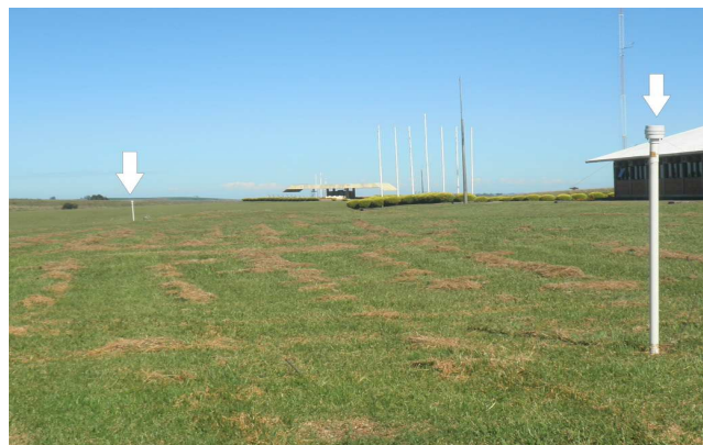
Figure 1: Inverted-V dipoles used in the interferometer installed in the Southern Space Observatory (SSO).
