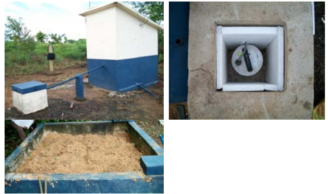
Figure 4 - View of the instruments and seismometer shelters of TUCA station (pictured above, on the left). Seismometer shelter internally lined by styrofoam plates (picture above, on the right) and seismometer pit covered with fine sand (bottom photo). The latter was covered with tile.
