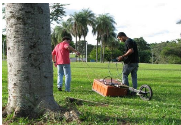
Figure 3 – Picture shows the GPR data acquisition in the proximity of a Guapuruvu with a 200MHz shielded antenna linked to a SIR-3000 equipment.
