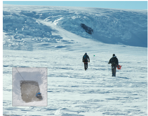
Figure 2. Laying bipole in central Transantarctic Mtns via harnessed, paired travel. Ti sheet metal electrode with high impedance buffer pre-amp shown in inset.
