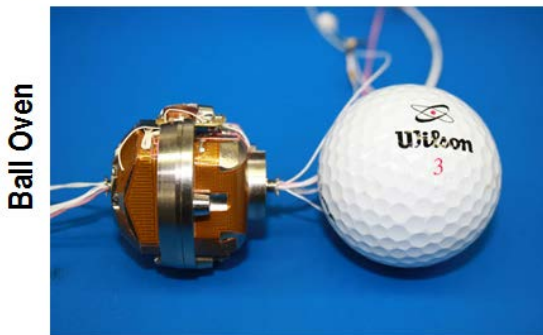
Figure 4. The GRAVILOG sensor ball and first stage oven
