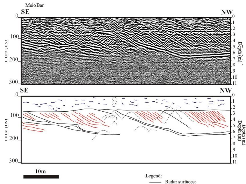
Figure 1.9 – GPR section of the Meio Bar in the Amazonas river.
