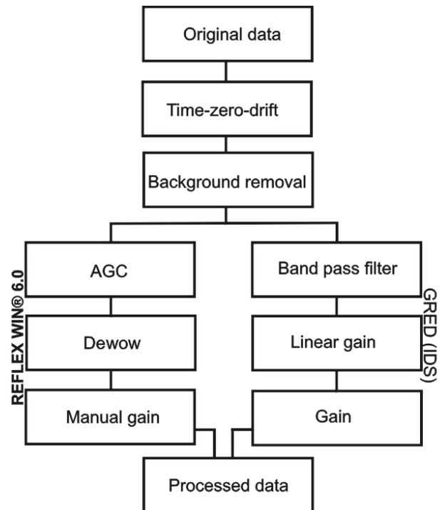
Figure 1.1 – Diagram of the data processing flow.
