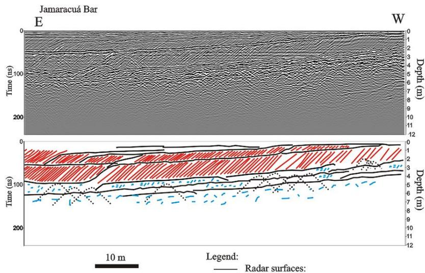
Figure 1.7 – GPR section of the Jamaracuá Bar in the Tapajós river.
