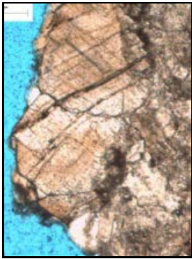
Figure 1. Thin section showing an intense fracturing. The sample corresponds to the upper part of the middle cretaceous interval
