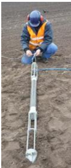
Figure 4: A SeisMovie™ piezoelectric source to be cemented down hole.
