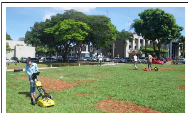
Figure 2: Geophysical survey performed after all the objects were buried.
