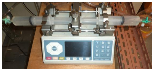
Figure 2. Programmable syringe pump (CHEMIX, Nexus 3000), operating at dual injecting-retrieving mode, by coupling two similar syringes onto a common driver (pusher).
