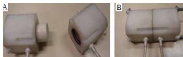
Figure 5. A jacketed plug sample and terminal chambers (A); Holding device when mounted and ready to measurements of the hydraulic resistance (B).
