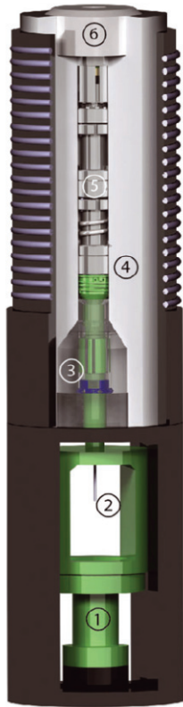
Figure 2. Sketch of the high-pressure triaxial testing apparatus (Paterson rig). After Madonna and Tisato (2013).
