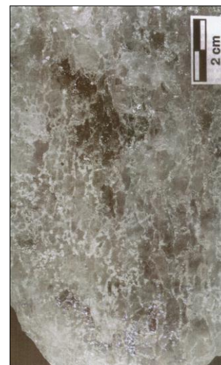
Figure 1: Halite from the Al Salif Diapir in Yemen showing vertical elongate grains due to flow in the diapir neck. Grain size approximately 1 cm and grain elongation ratio 1:3. P wave anisotropy in single crystals reaches up to 7% and s wave anisotropy can reach 16% which produces shear wave splitting.
