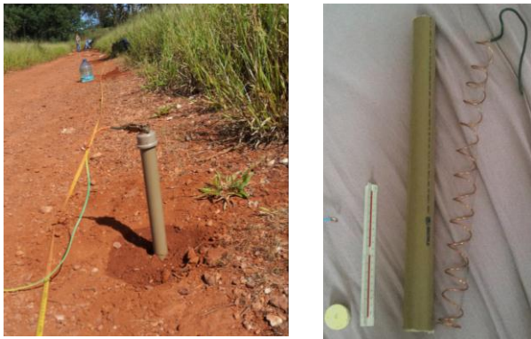
Figura 4 – Cu-CuSO 4 electrodes made for this survey.
