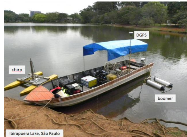
Figure 2: A small boat with a boomer and a double chirp at Ibirapuera lake, São Paulo city. IPT, 2011a.
