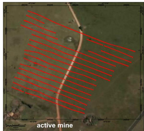
Figure 4 - Localization of measuring stations. There were 955 simultaneous measurements of radiometry and magnetic data, with an interval of 5 m along the profiles. The region without reading at the time the survey was flooded.
