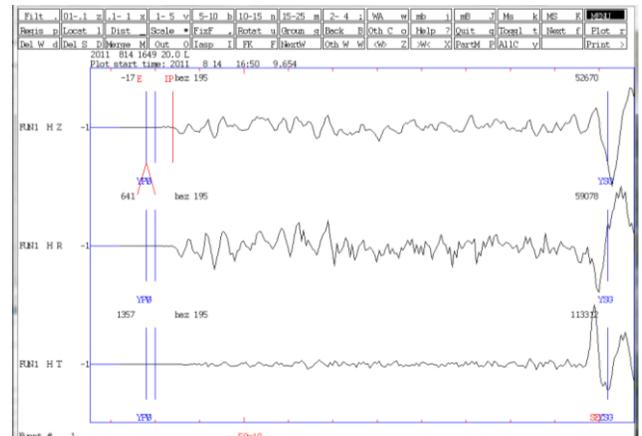
**Figure 7:** Seismogram of the Ijaci event on 14/08/2011, with horizontal components north-south and east-west directions rotated to radial (HR trace, center) and tangential (HT trace, bottom). The back azimuth is 195 degrees, so the horizontal components rotated 15 degrees clockwise. Note the clarity of the S phase in the tangential component.
