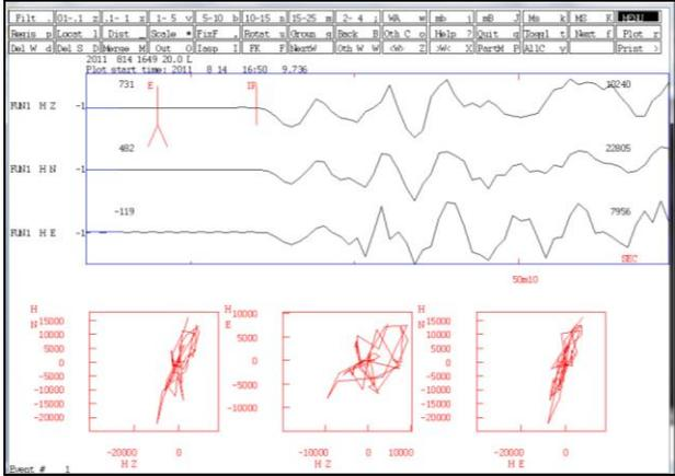
**Figure 4:** Seismogram of Ijaci event of August 14, 2011 in the vertical, norte-south and east-west directions (three above traces) and particle motion in the north-south x vertical, east-west x vertical and horizontal (north-south x east-west) directions. Observe that the event-back azimuth in the lower right figure is approximately equal to 195 degrees.
