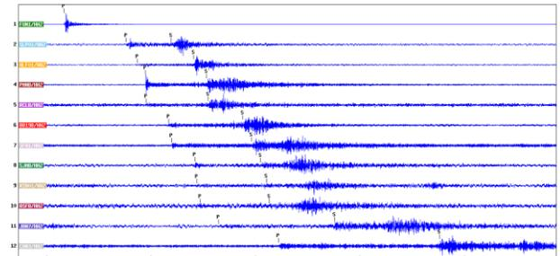
**Figure 3:** Seismogram of Ijaci main event of August 14 of 2011 (vertical components) in the twelve stations of Figure 2. Also shown are the markings of the P and S phases in order of increasing arrivals.
