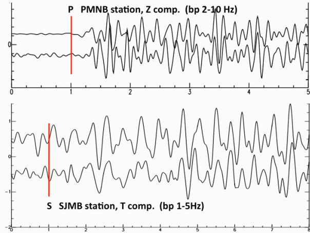
**Fig. 3.** Example of cross-correlation of P and S waveforms at stations PMNB and SJMB. Top trace is the 19-May (mainshock), bottom trace is the 12-September (master event). Vertical lines show the picked arrival times. Horizontal scale is in seconds.
