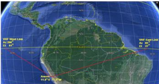
Figure 2. Projections of the Ancon 250-MHz SCINDA ray paths onto the Google Earth map of South America.
