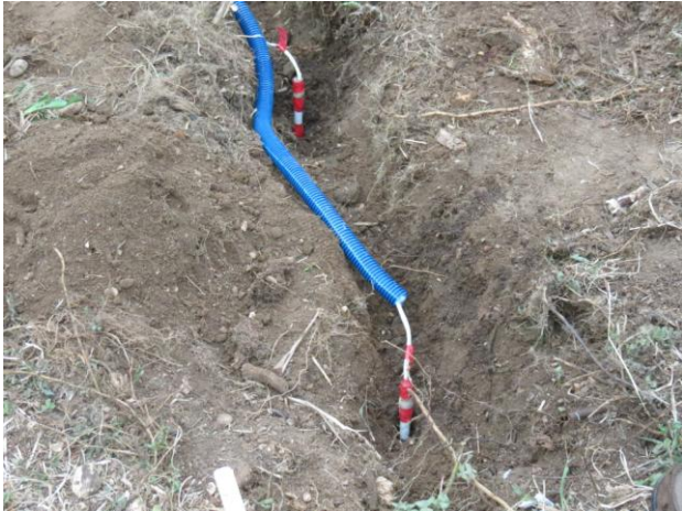
Figure 3 - Electrodes placed in the experiment area.
