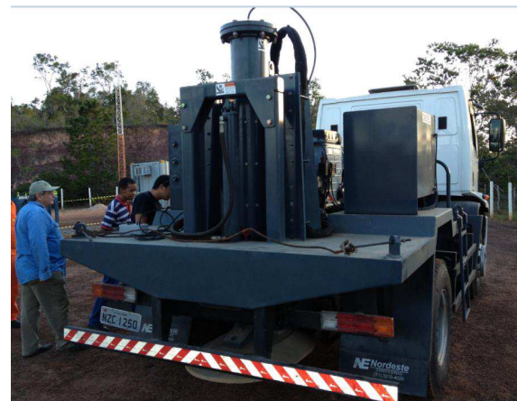
Figure 2. The AWD AF-450 – Accelerated Weight Drop source used in the experiment.
