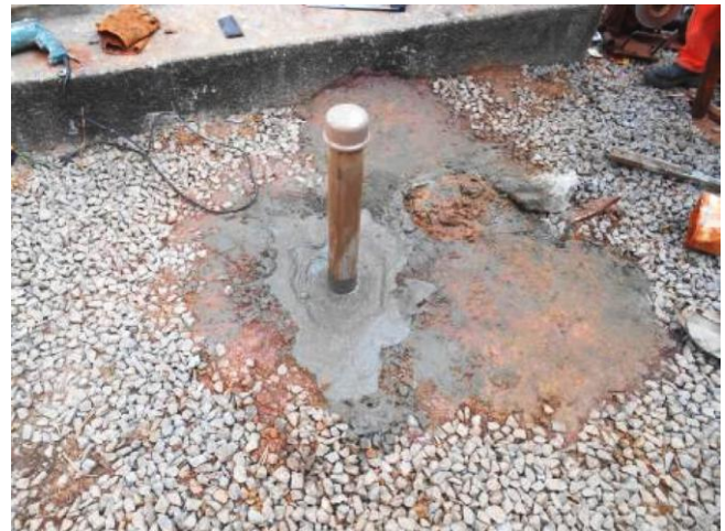
Photo 1 - Detail of the borehole for PS testing.
