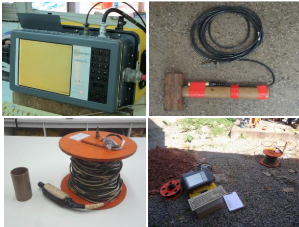
Photo 2 - Geophysical equipments used for the PS test: seismograph (above, on the left); sledgehammer with trigger switch (above, on the right); triaxial borehole geophone (below, on the left); equipments in the site (below, on the right).
