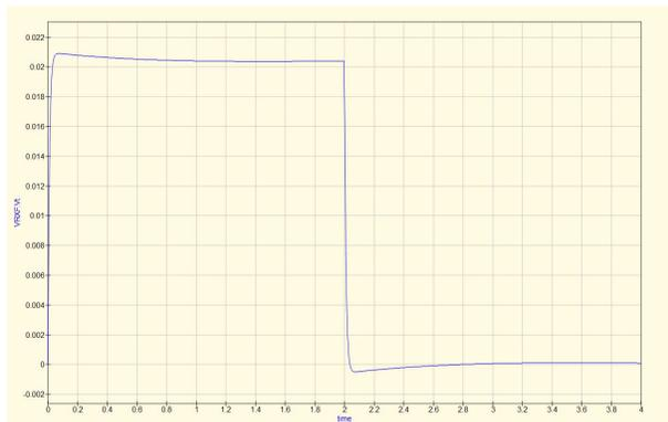
Figure 19: RLC circuit response  $L = 1800\mu H$
