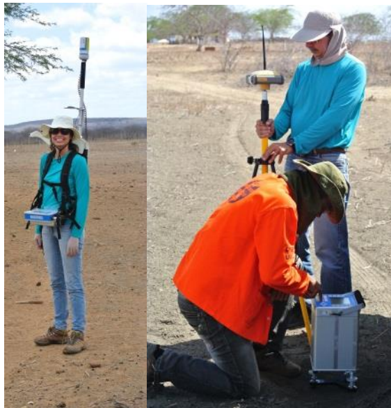
Figure 8. Magnetic and gravity data acquisition.
