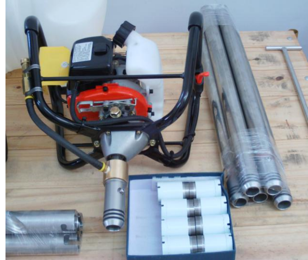
Figure 3 – Portable core extractor used to obtain in situ rock plugs on outcrops.
