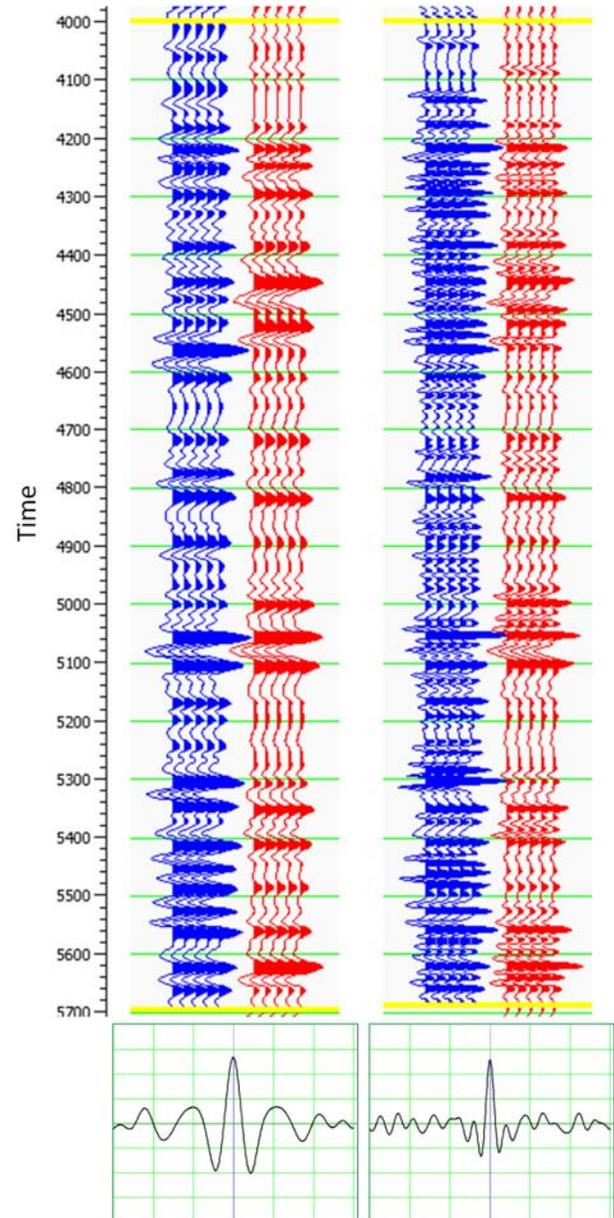
Figure 7 – Well-seismic correlations for normal bandwidth and broadband data. The synthetic traces calculated from the well logs are in blue, and the composite seismic traces are in red. The bottom plots show the correlation between the well and the seismic data. The left track shows the normal bandwidth, and the right plot shows the broadband data.
