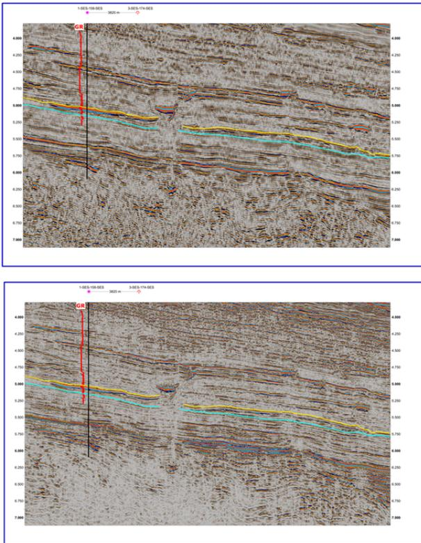
Figure 8: Conventional pre-stack depth migration converted to time (top) and broadband pre-stack depth migration converted to time (bottom) with sequence stratigraphic interpretation and gamma ray log for Barra 1-SES-158 well.
