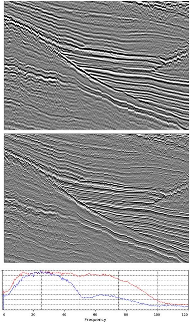
Figure 5 – Seismic sections before (upper) and after (lower) broadband processing. The spectra show the normal bandwidth data in blue and the broadband data in red.
