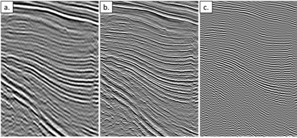
Figure 4: Seismic sections displaying various bandwidths. Panel (a) is deficient in high frequencies making the section blurry. Panel (b) is the full bandwidth section. Panel (c) is deficient in low frequencies making the section appear “ringy”.
