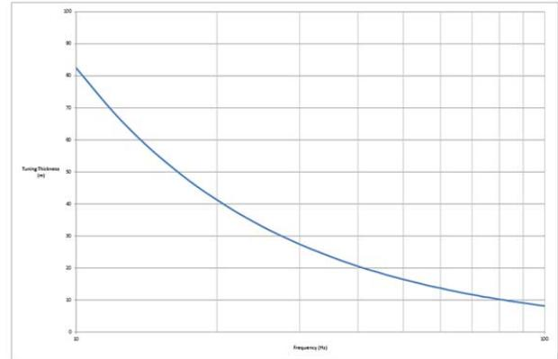
Figure 3: Tuning thickness vs. Frequency (3,400 m/s)
