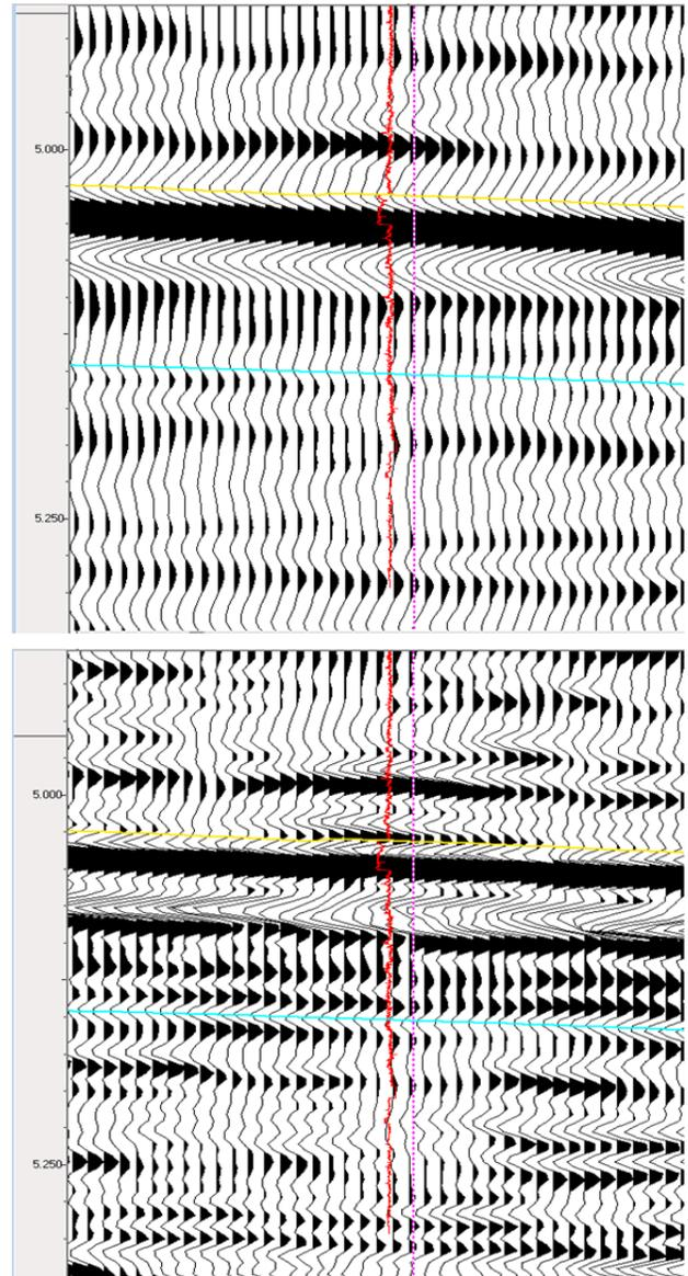
Figure 9: Zoom of conventional PSDM (top) and broadband PSDM (bottom) both converted to time with gamma ray log and sequence stratigraphic interpretation.
