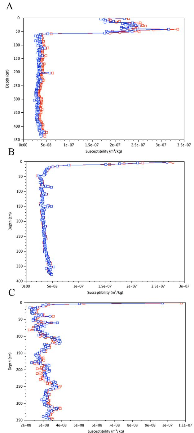
**Figure 2:** Magnetic susceptibility with depth for Cores PT-03 (A), PT-04 (B) and PT-06 (C). Red color represents magnetic susceptibility at frequency 976 Hz and blue at frequency 15616 Hz.
