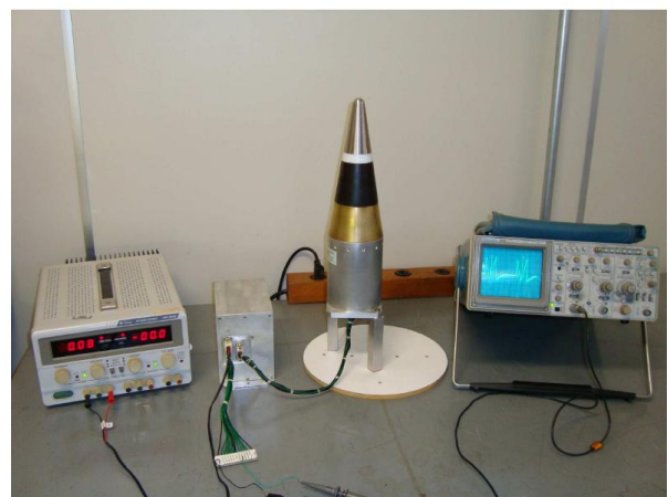
Figure 1: Langmuir probe used during the launches being tested and calibrated in the laboratory.
