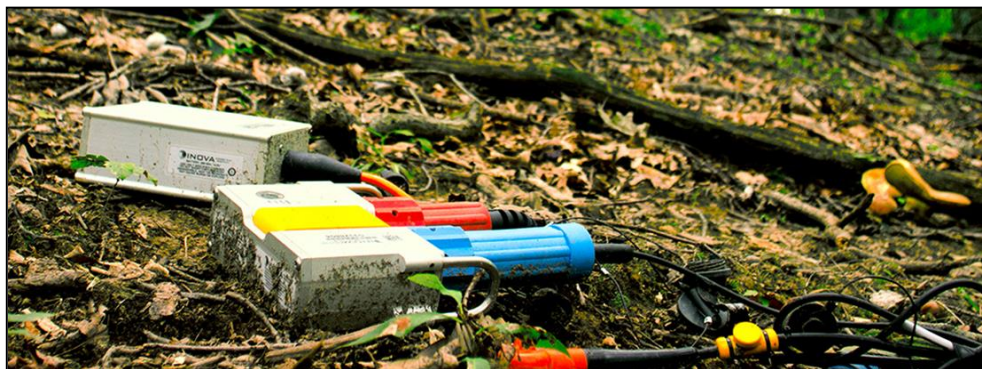
Figure 2 shows a compact cableless node with a connected battery and 3C sensor.
