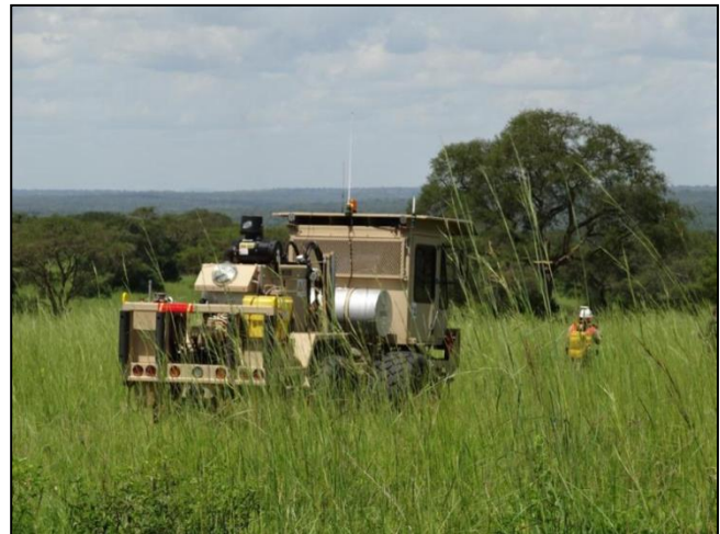
Figure 1 shows a small sized vibrator working in a national park in Uganda. Picture courtesy of
