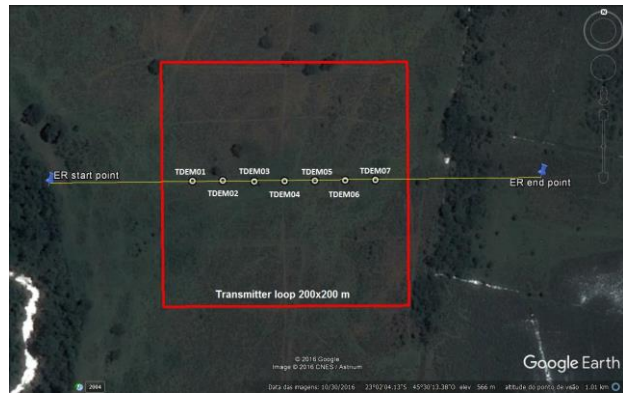
Figure 5. Data acquisition points in Taubaté city. The blue points show the starting and ending points of the ER imaging with 400 m length. The red square is the TDEM transmitter loop with 200x200 m and the points inside de loop (TDEM01, TDEM02, ... TDEM07) are the TDEM acquisition points with 25 m spacing.
