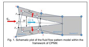
where  $p_{top}$  and  $p_{bot}$  are the pore fluid pressures on the top and bottom faces of the crack, as depicted in Fig. 1, and  $c_{top}$  and  $c_{bot}$  are leak-off coefficients, which are
