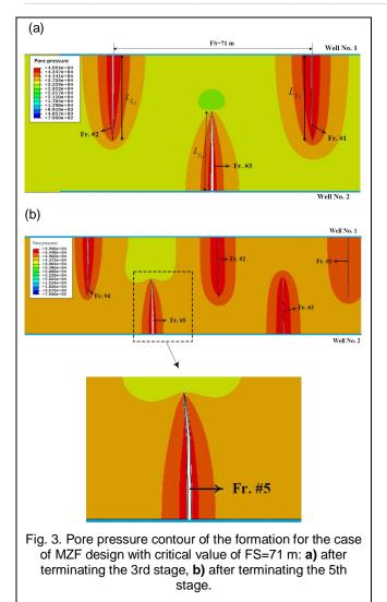
through non-uniform fracture spacing. The critical value of the FS between Fr. #2 and Fr. #5 has been determined as 105 m so that the Fr. #5 propagates in a straight path, as demonstrated in Fig. 4. By comparing Figs. 3 and 4, one can see that the pore pressure of the formation declines as the FS increases.
